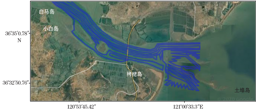
图 2 测线布设 Fig.2 Schematic diagram of the surveying line layout
